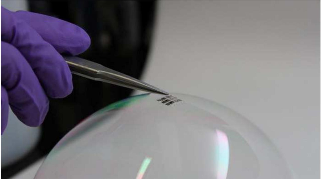
Researchers at MIT have created prototype solar cells so light and so thin, that they can be balanced on the surface of a soap bubble without breaking it (Credit: Joel Jean and Anna Osherov)
