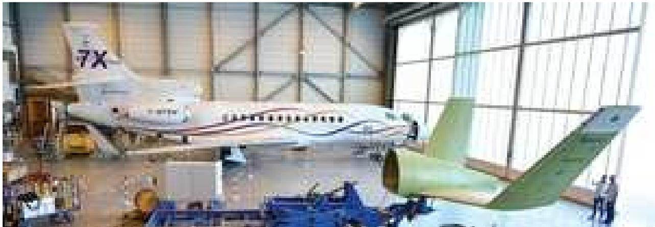
**A full-scale U-tail was positioned behind the Falcon 7X to assess shielding of real engine noise. Credit: Clean Sky**
