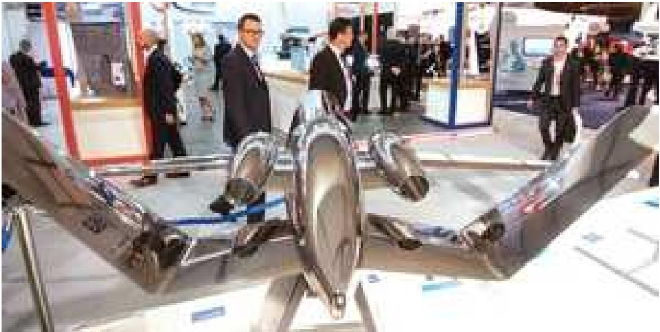
The business jet wind-tunnel model evaluated U-tail and low-sweep laminar flow wing.
