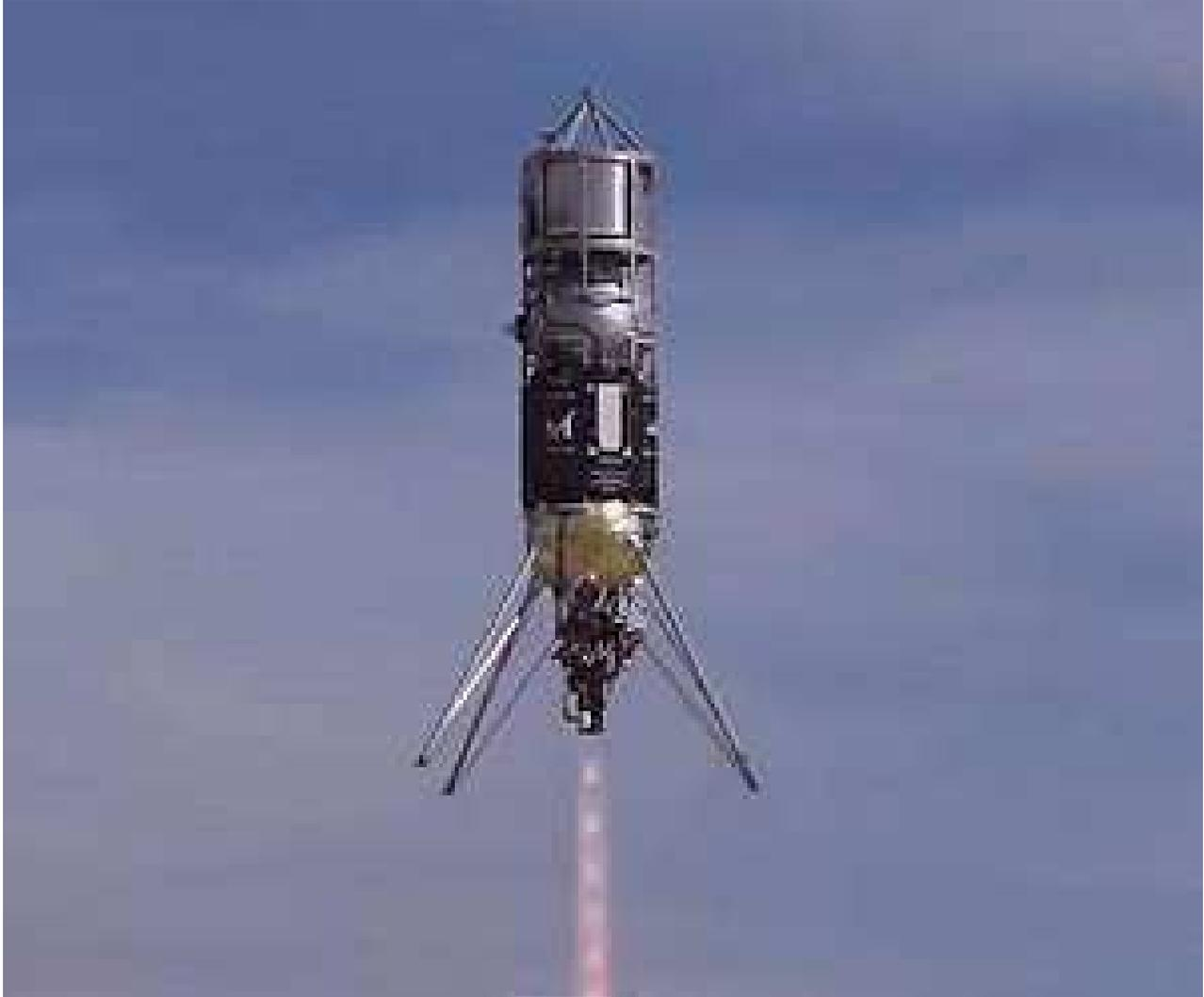
**A rocket flying several landing technologies was recently flown in the Mojave Desert. These flight tests, coordinated by NASA, are helping to develop technology for precise landings in uneven terrain. Image Credit: NASA/JPL-Caltech.**
