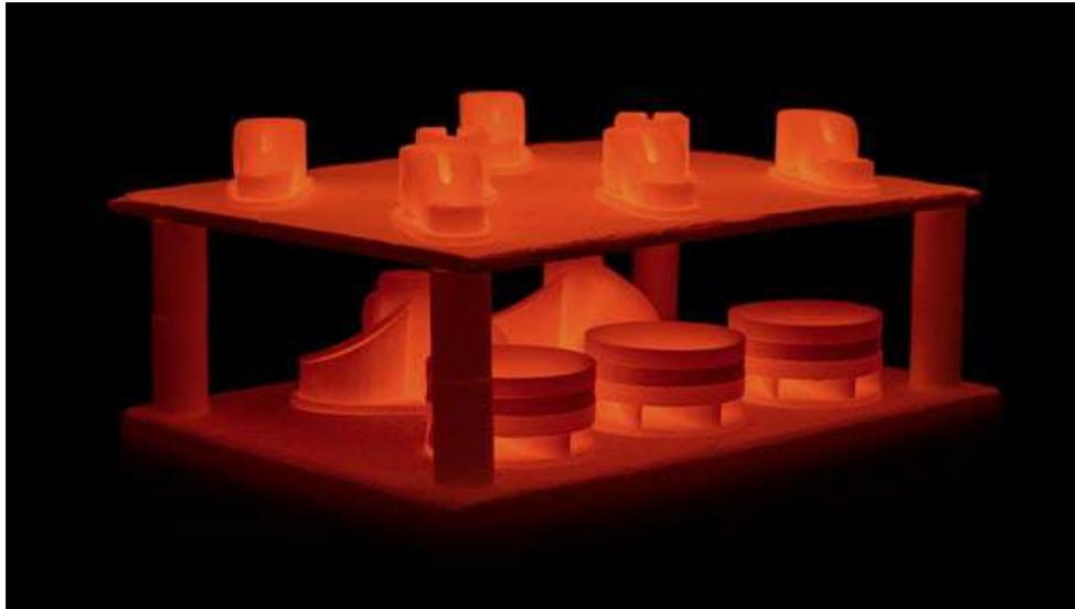
Sintering Multiple Parts – Desktop Metal’s Studio System includes a fully-automated, office-friendly sintering furnace with fast cycle times and a peak temperature of 1400°C, allowing for the sintering of a wide variety of materials. (Credit: Desktop Metal)
