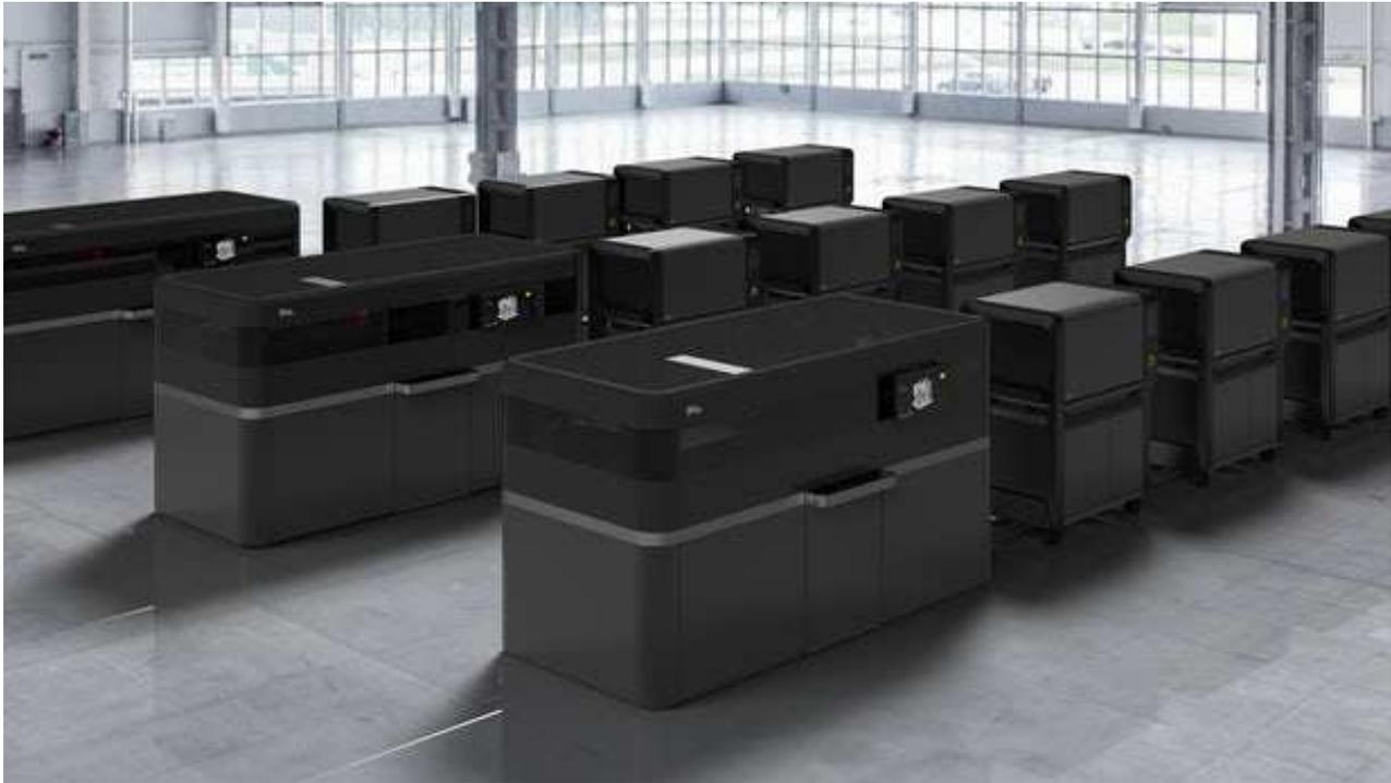
The rest of the process – de-binding and sintering – looks much the same as the Studio system. Print resolution is as fine as 50 microns, roughly the width of a human hair. And while no final pricing has been given yet on the full system, each printer will retail for around US\$360,000.
